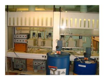
The laboratory and pilot scale mixer-settler units are available in flow (org+aq+recycle) ranges from 50 to 500 l/h.
