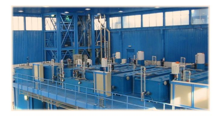
The industrial mixer-settler units are available in flow ranges (org+aq+recycle) from 500 l/h and upward.
