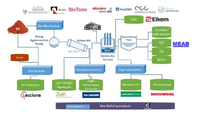
The figure demonstrate the production of REE concentrate, Ga concentrate, alumina/soda solution and rutile concentrate from the hydrometallurgical processing of engineered slags/sinters produced in RemovAL pyro-metallurgical pilot plants. Ga is co-extracted both from the slag and the Bayer liquor. At least 500 kg of slag and 100 l of Bayer liquor will be processed at **MEAB** solvent extraction pilot plant in Germany.
